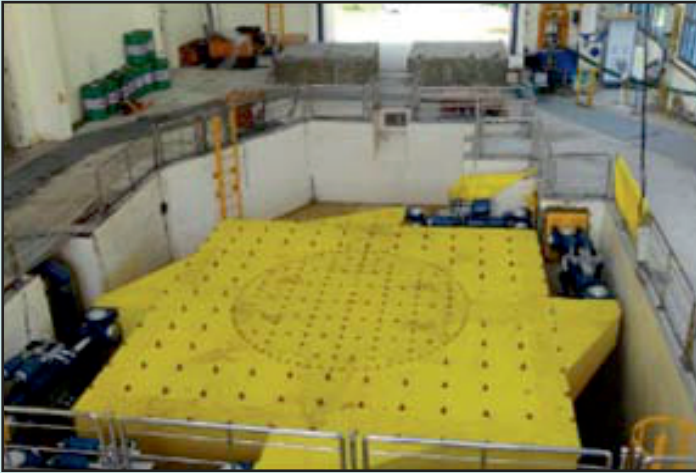
100 Tonne shake table for seismic studies, IGCAR
